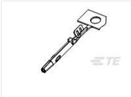
TE 产品编号1418971-1 CENTER CONTACT, PLUG
