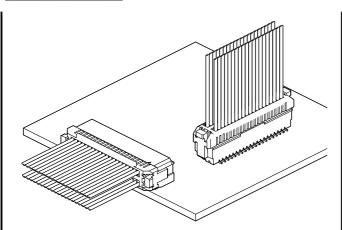
Developed for PDP, LCD or small electronics equipment. This is a dual-row small crimp type connector with a secure locking system or without-designed for different applications. The PC board layout is compatible with that of existing SHD connector, which allows for replacement of the above existing connector.
