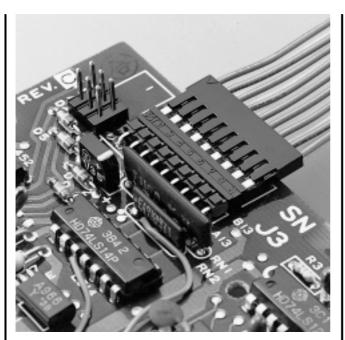
The RE series was developed as a reliable, low-cost, crimp style connector for connecting wires to printed circuit boards. It is well suited for completing the internal connections of office automation equipment, such as personal computers, office computers, and their peripheral devices.
