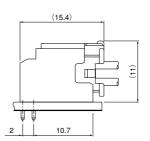
Note: 1. The above figure is the figure viewed from the connector mounting side.
