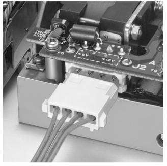
This reliable, low cost connector is suited for bringing power to printed circuit boards in office automation equipment. A major application has been in secondary power supply circuits of floppy disk drives.
