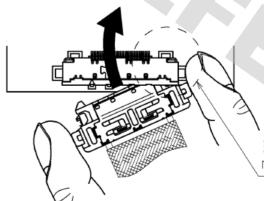
In case connector is withdrawn with lock that is locked on one side. mate the plug again and withdraw with <Correct withdrawal> method.
