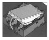
③ The reinforced lock is also released and the un-mating is complete
