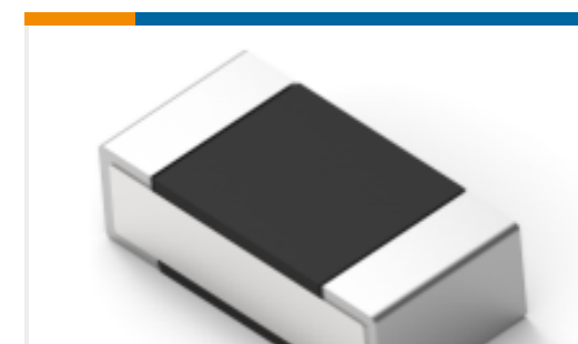
TE Part #2-2176308-0 RP 1E 0.1W 210K 0.1% 25PPM 5K RL
