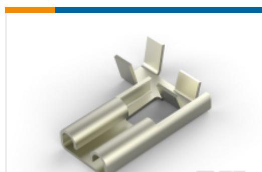
TE Part #280050-3 250 FASTON, FLAG, REC., 16-20 AWG, NPST
