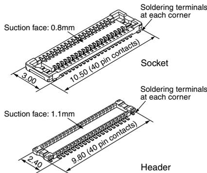
3. Low profile and highly resistant to various environments possible with the use of highly reliable **“TOUGH CONTACT ADVANCED”** connector design.
