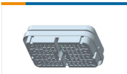
TE Part #1-2112162-1 21POS,TAB 2.8X0.8,TAB HSG,SEALED ASSY
