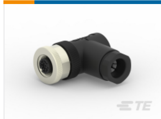
TE Part #T4112002081-000 M12,FEMALE,RA,A CODE,8P,PG9, GOLD
