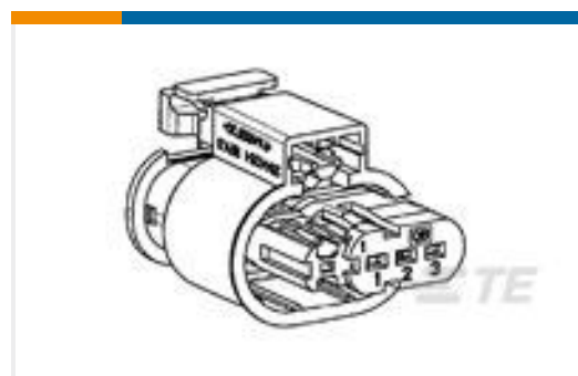
TE Part #284556-1 2 POS. CONN. FOR SPARK COIL
