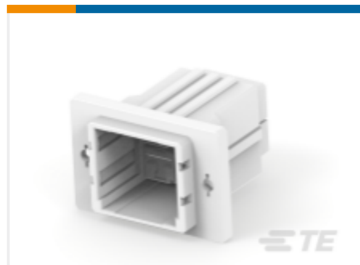
TE Part #1-353046-3 Receptacle and Tab Housing: 5.08 or 10.16 mm pitch, 250-600V
