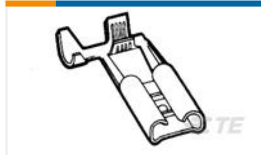
TE Part #280050-7 250 FASTON, FLAG, REC., 16-20 AWG, TPPB
