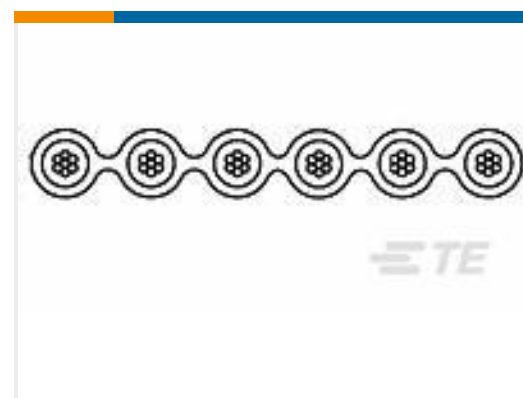
TE Part # 1-167019-0 10P. RIBBCBL 28AWG P1.27
