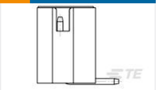
TE Part #1775317-7 HPI.,2.5MM PITCH,V/T,SMT TYPE,7 POS
