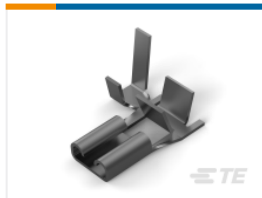
TE Part #63316-5 187 FASTON FLAG REC 18-14 AWG TPBR
