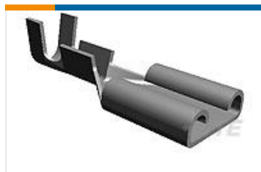
TE Part #42617-2 187 FASTON REC 20-16 AWG TPBR
