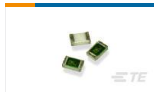
TE Part #8-1676481-6 CPF 0603 30K 0.1% 25PPM 1K RL
