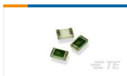
TE Part #5-1614882-1 CPF 0603 16K 0.1% 25PPM 5K RL
