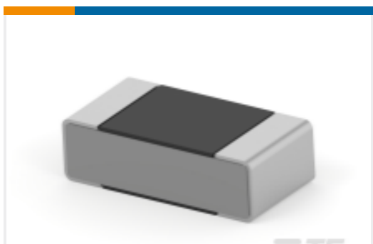
TE Part #2176280-7 CPF 0402 115K 0.1% 25PPM 1K RL
