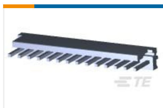
TE Part #1-640251-4 3.96mm Wire-to-board housing: receptacle, no mating alignment, SL 156
