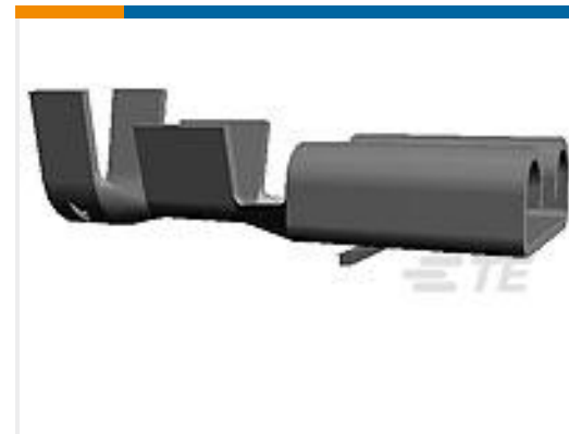
TE Part #1217281-2 FF 110 REC 24-20AWG TPBR
