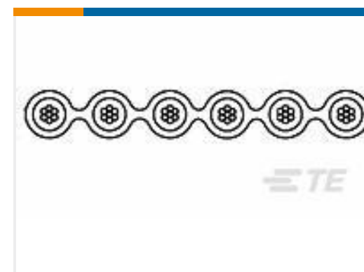
TE Part # 1-167019-4 14P. RIBBCBL 28AWG P1.27
