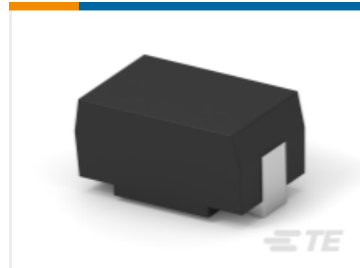
TE Part #6-1879022-9 SMD Power Resistor: 7 Watt, 200-2M Ohm
