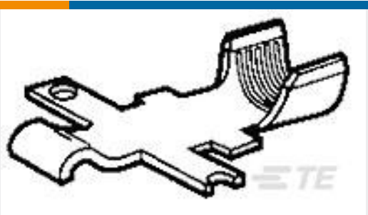
TE Part #53880-2 CONTACT,PWR LK,SRS2,STRIP,CRMP
