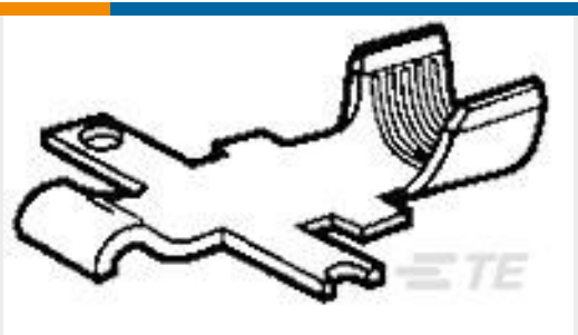
TE Part #53880-4 CONTACT,PWR LK,SRS2,LS PC,CRMP
