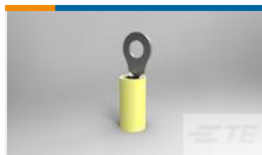
TE Part #696424-6 TERMINAL,PIDG PVF2 R 12-10 10
