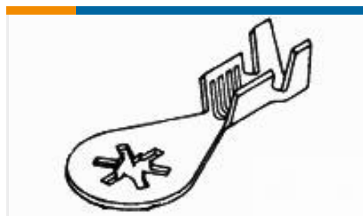
TE Part #640204-1 RING .164 (4.17 MM) 22-18 AWG TPST
