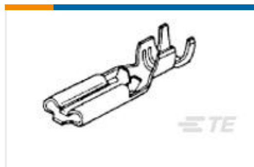
TE Part #175412-1 PL 110 REC 24-20 AWG 0.25 X 10.4 PTBR
