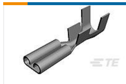
TE Part #170213-2 250 FASTON, REC., 18-14 AWG, TPBR
