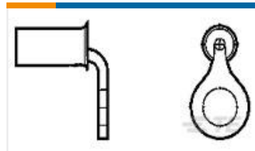
TE Part #55654-1 TERMINAL R 90 DEG PG 8 10
