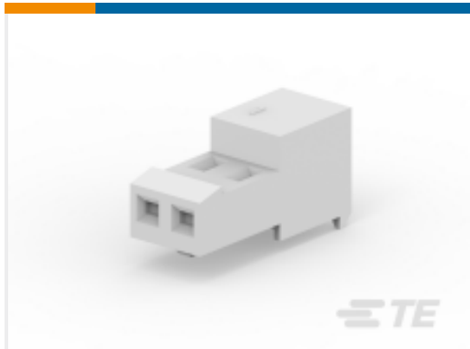
TE Part #3-641534-2 Nylon Tin Plated Receptacle: 2.54mm, No Mating Alignment, MTA 100
