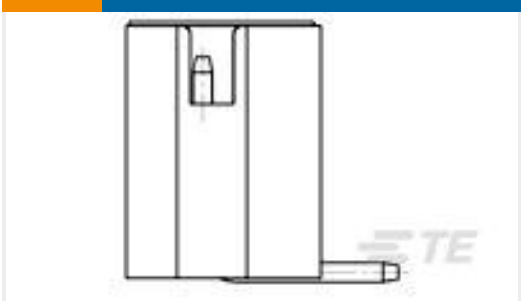
TE Part #1775470-5 HPI CONN., 2.0MM, V/T, SMT, 5P, 80U"
