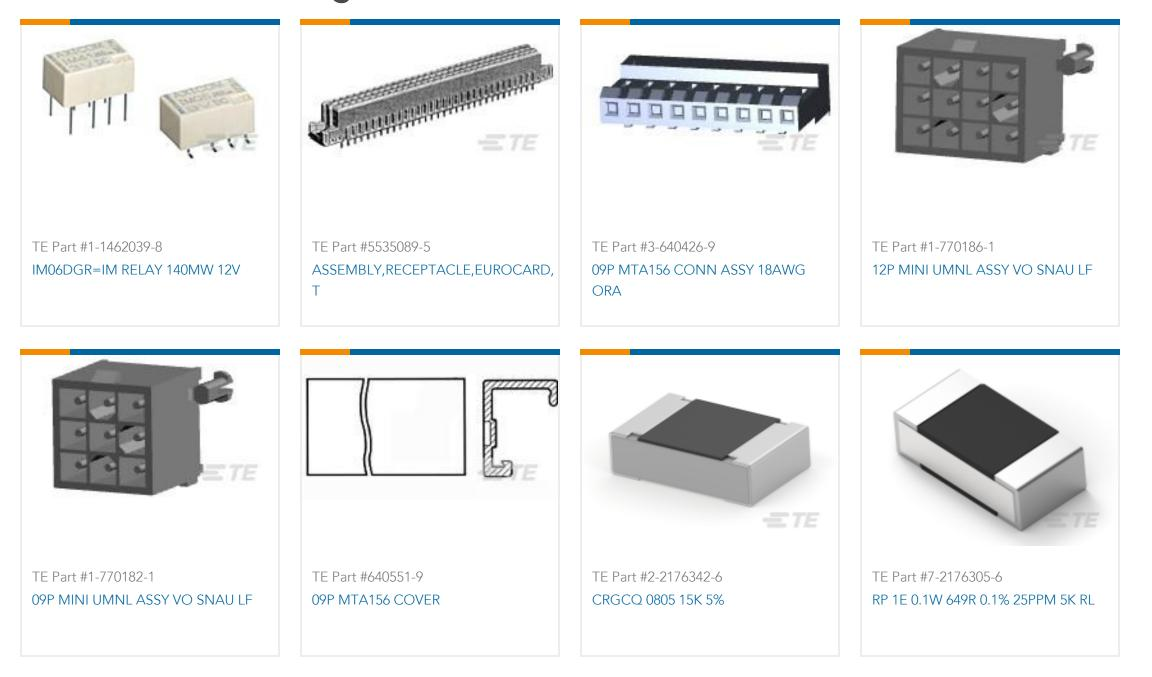
Eurocard Connectors, Receptacle, Board-to-Board, 32 Position, .1 in [2.54 mm] Centerline, Printed Circuit Board, 2 Row, Vertical, Eurocard Type B
