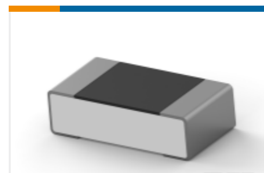
TE Part #1-2176369-6 RQ 0603 57R6 0.1% 10PPM 5K RL
