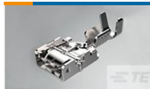
TE Part #336076-5 250 FASTON,E SPRING REC.,17-14 AWG,PNST
