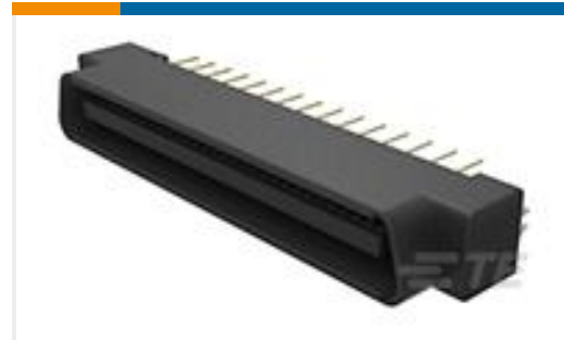
TE Part #1734100-7 Champ050 series,68pos,Au over PdNi
