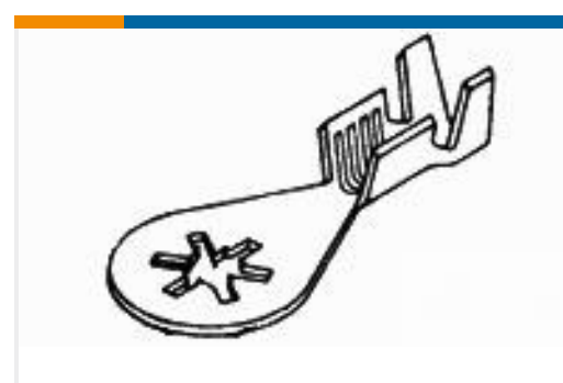
TE Part #640051-1 RING TONGUE .164 18-14 AWG SST
