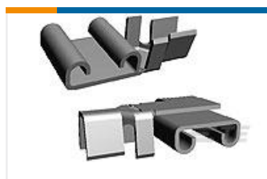
TE Part #61188-1 250 FASTON FLAG REC 16-12 AWG TPBR
