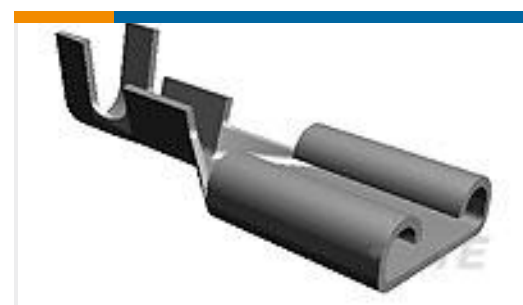
TE Part #42400-1 250 FASTON REC 18-14 AWG BR
