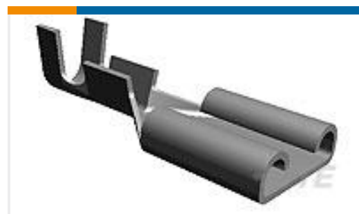
TE Part #42510-1 250 FASTON REC 22-18 AWG BR
