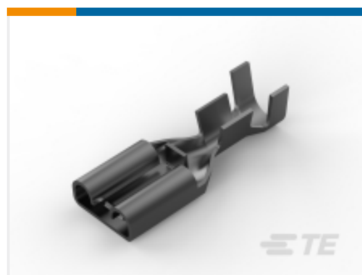
TE Part # 63854-2 250 PL MKIII REC. 18-14AWG TPBR
