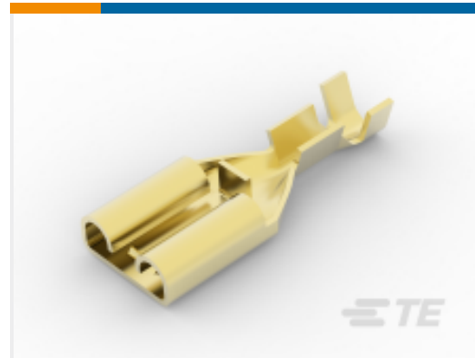
TE Part # 63933-1 PL .250 TERMINAL REC 22-18 AWG BR
