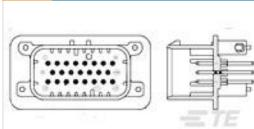
TE Part #1-776228-1 23POS,PIN DIA 1.3,HDR ASSY, 180DEG,COD 1
