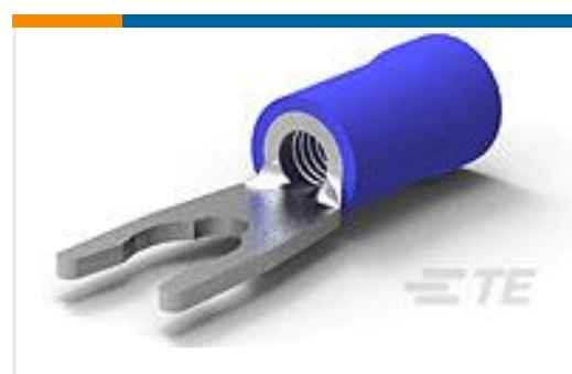
TE Part #53244-2 TERMINAL,PG SPR SPD 16-14 8
