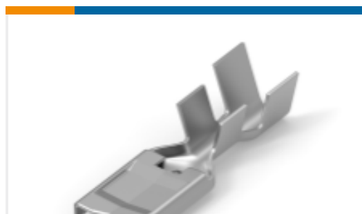
TE Part #520982-2 ULTRA POD: Straight, Receptacle Assembly, Tin Plated, .187 inch
