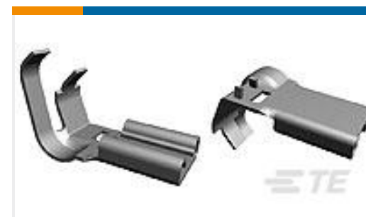
TE Part #42404-1 250 FASTON FLAG REC 18-12 AWG NPST
