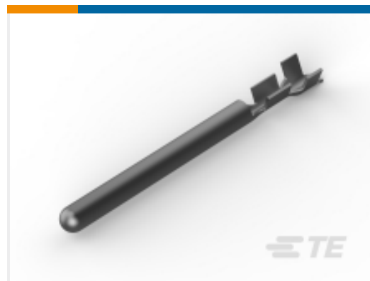
TE Part # 62358-1 PIN .080 (2.03 MM) 24-20 AWG TPBR
