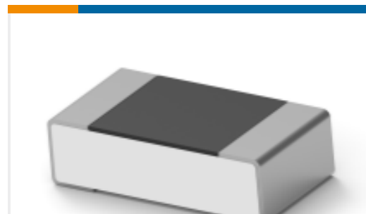
TE Part #2176371-3 RQ 0603 4K87 0.1% 10PPM 5K RL
