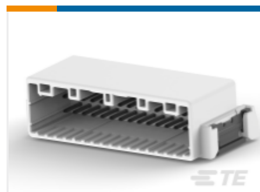
TE Part #2237138-1 32POS,TAB0.64X0.64,HDR ASSY, 90DEG,SMD
