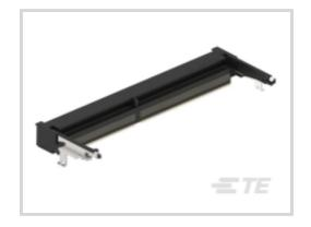
DRAM Type: Small Outline (SO) Stack Height: 8 mm [.315 in ] Module Orientation: Right Angle PCB Mounting Style: Surface Mount Connector System: Cable-to-Board
